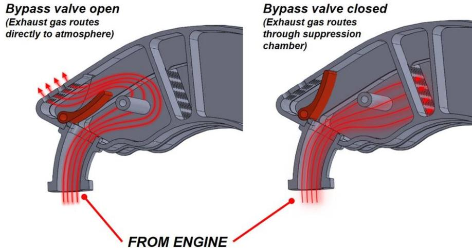
Figure 6. Exhaust system bypass valve. Shown in 'OPEN' and 'CLOSED' positions.
