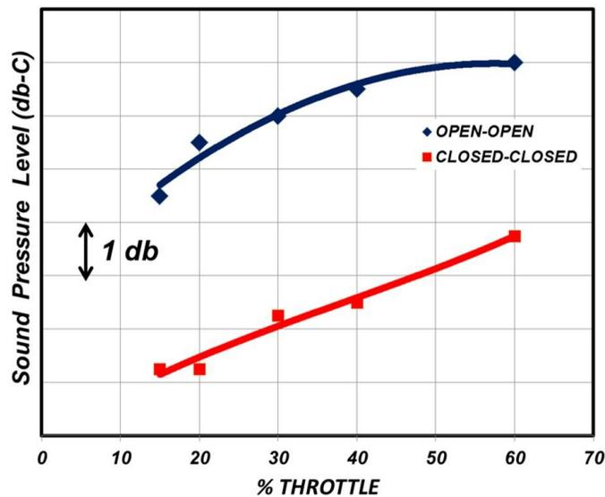
Figure 9. Noise reduction along a 16-14 propeller curve.
