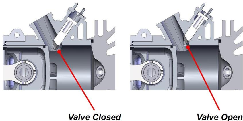
Figure 5. Variable exhaust port valve.
