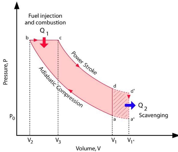
**Figure 4. Ideal engine cycle for two-stroke engine with variable exhaust valve.**
