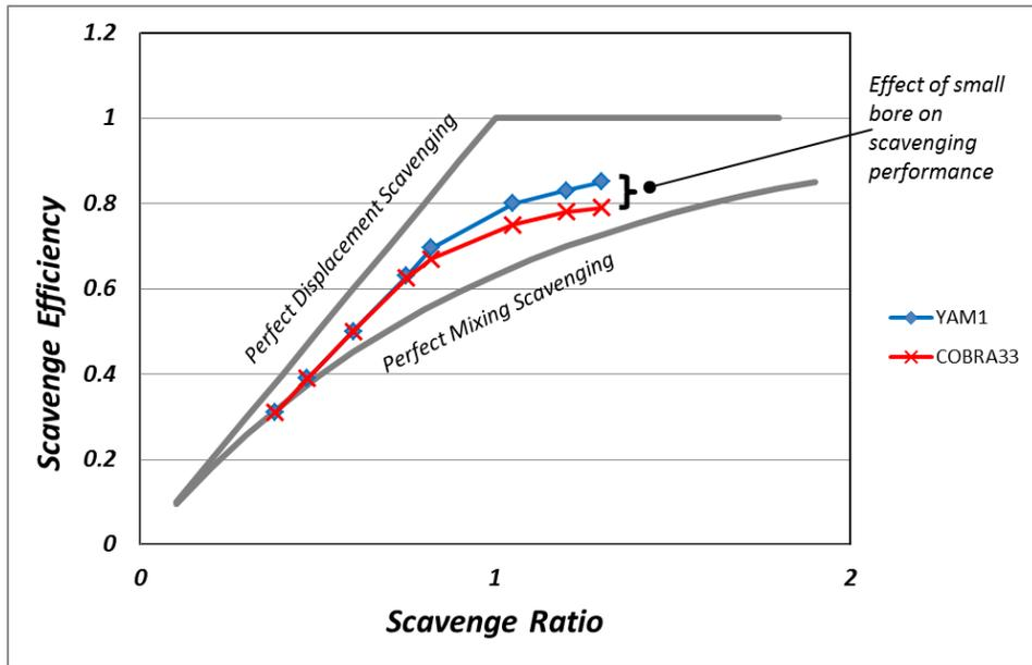
Figure 3. Scavenging model used in simulation.
