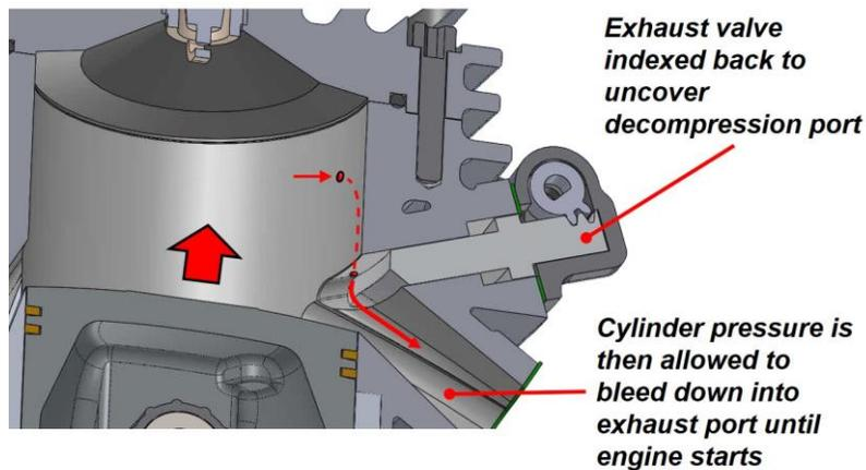
Figure 10. Engine cross section showing exhaust port valve used as decompression device.
