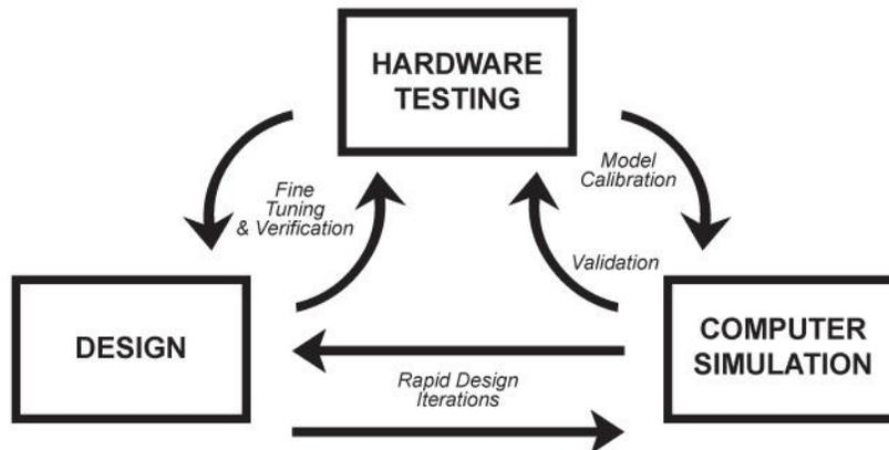
**Figure 2. Iterative hardware development process.**
