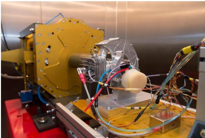
**Figure 1. Test cell installation. This figure shows an eddy current motoring dyno installed in a temperature controlled test environmental cell (-30F – 150F range).**
