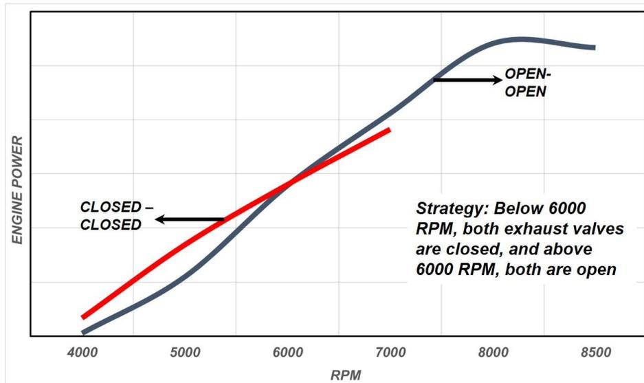
**Figure 7. WOT Power output under both CLOSED-CLOSED and OPEN-OPEN configurations.**
