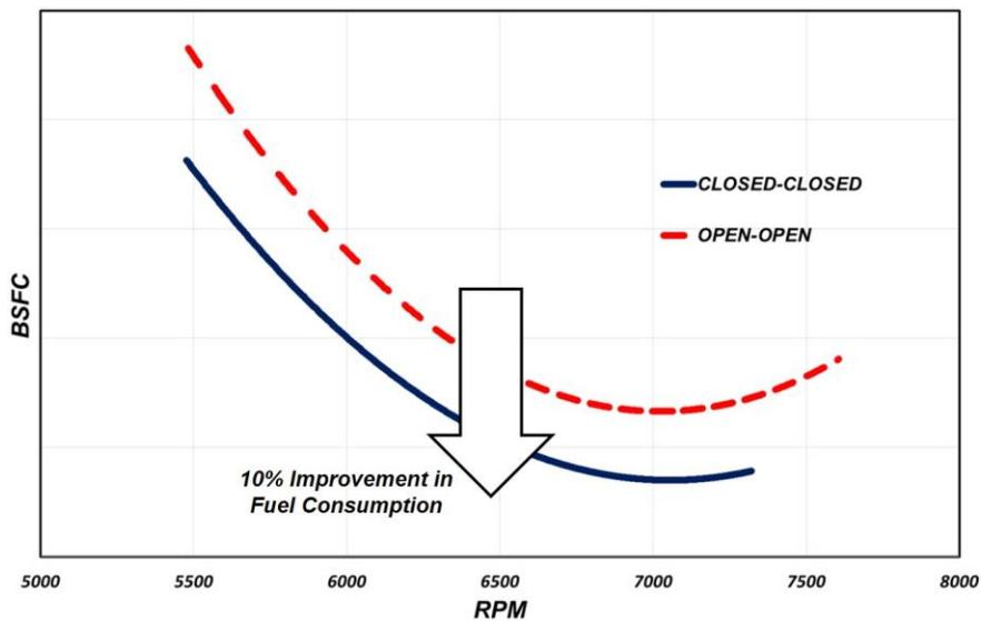
**Figure 8. Fuel consumption improvement along a 16-14 propeller curve.**
