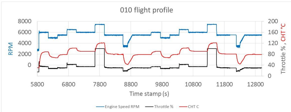
Figure 4: Engine 010 flight profile data
