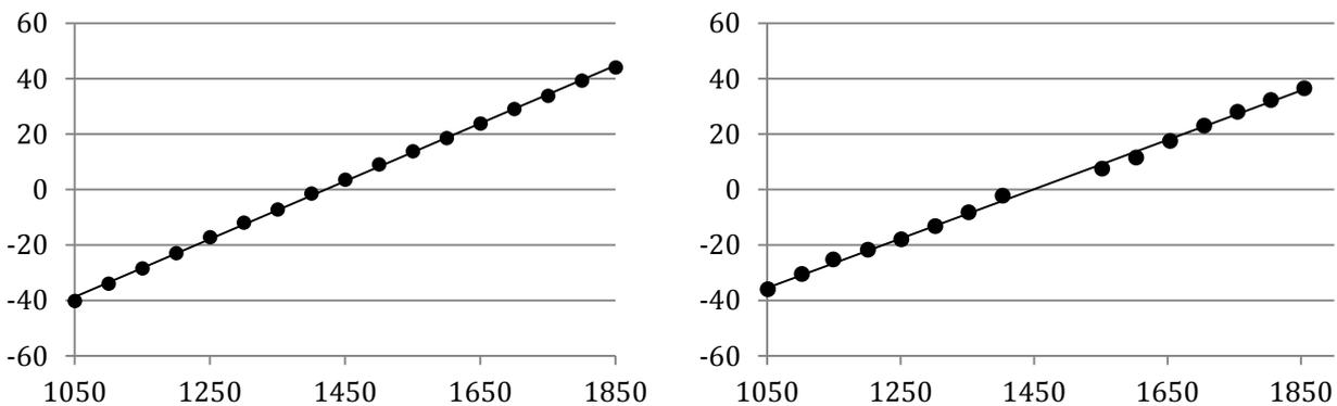
**Figure 2 Feedback position v. angle, at zero hours (left), at 575 hours (right)**
