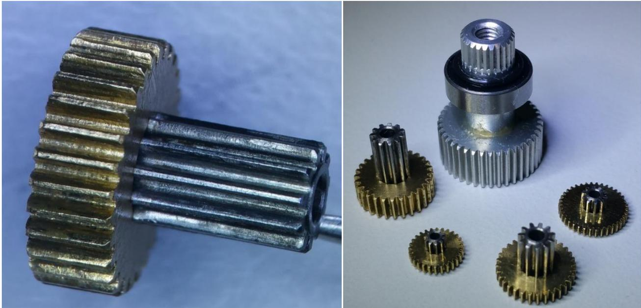
**Figure 3 Gear showing wear on flanks (left), inspection of all gears (right)**
