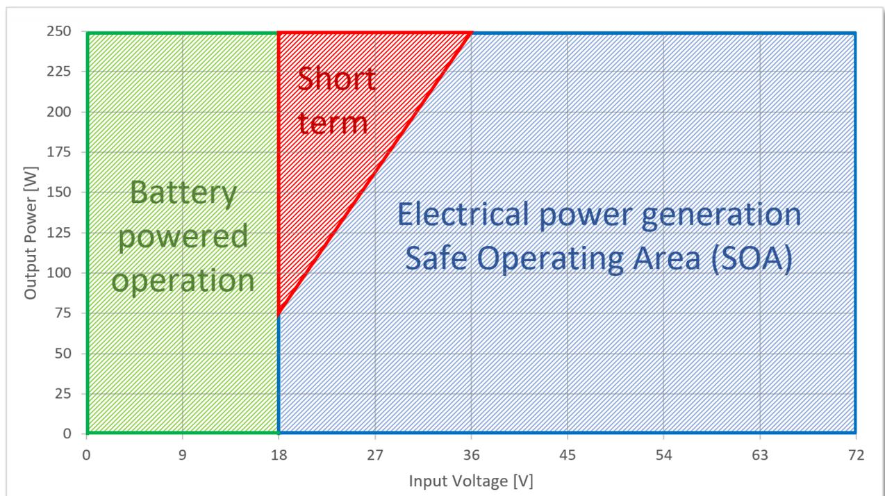
Graph 1 – Safe Operating Area (ambient temperature +25°C, fan fitted and running)
